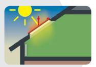
External accessories offer the best protection from high temperatures. They absorb UV radiation, protect the external glazing and keep warm air
