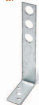
To achieve the recommended safe working loads use 30 x 3.75mm sherardised square twist nails in all pre-punched holes, together with M12 HT bolts where required.
